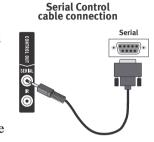
Control Out-Serial connector (the upper mini jack) on the back of the DVR.
