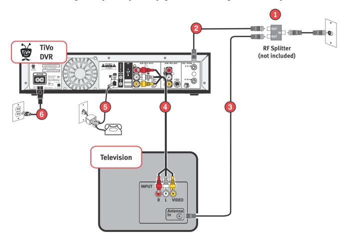
This setup works best if your TV program source is antenna or cable with no cable box, and you have a TV with more than one input.
