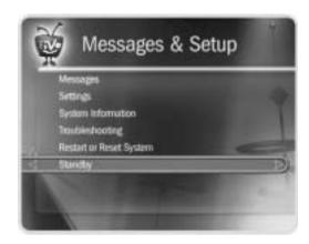
If you used only RF coaxial cables to connect your program source (antenna or cable) to the DVR, and also to connect the DVR to your TV, Standby mode allows RF signal pass-through. This means you can watch channels on your RF program source using your TV's tuner instead of the DVR's tuner—and that means you can watch one channel while recording another! Keep in mind, you won't have DVR functionality in live TV (pause, rewind, etc.) while the DVR is in Standby.
